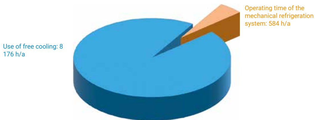
Fig. 1: The refrigeration system of a Slim Line Q15 air-conditioning unit operates for just under 7% of the total annual operating time.
