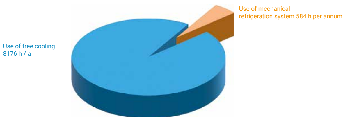
Fig. 1: The refrigeration system of a Slim Line Q15 air conditioning unit is used during about 7% of its service life.
